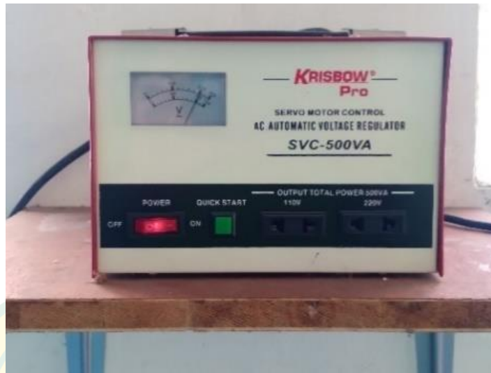
Gambar 3. 4 Automatic Voltage Regulator
