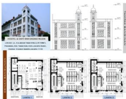
Figure 3. Proposed design of dasaad musin as a new function (Hostel and Cafe).
