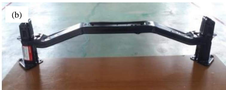
Figure 1. Crash box and bumper beam assembly : (a) assembly diagram; (b) assembly spare part; (c) spare part number.
