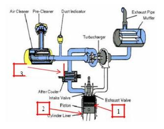
Fig. 4. Air intake system
