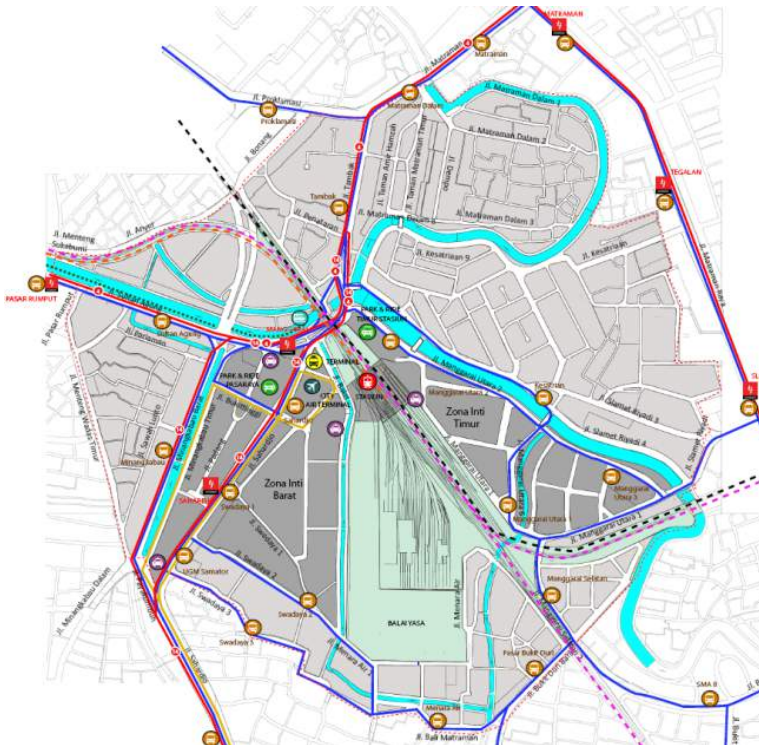
Figure 12: The possibility of the pedestrian ways and bikers' ways which will be proposed in Mangarai District to apply the concept of Transit Oriented Development Source: Dinas Tata Ruang DKI
