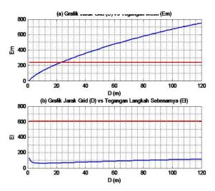
**Fig. 5.** (a) Effect of Grid Distance on Em, (b) Effect of Grid Distance on El
