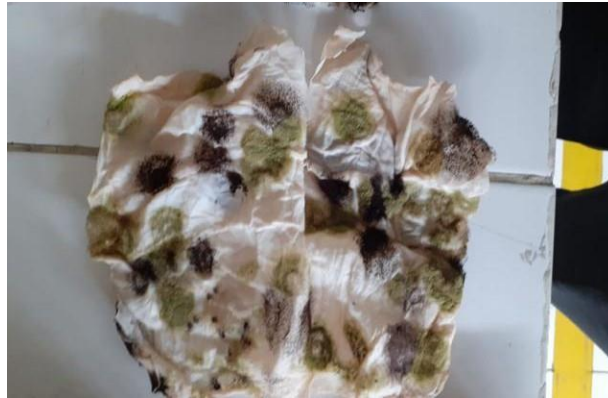
Figure 12. Biocellulose which is dried with large water content with released water content (80.82%)
