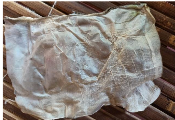
Figure 13. Biocellulose which is dried with large water content with released water content (91.32%)
