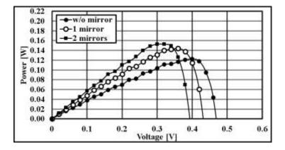
Figure 9. The P-V curve of solar cell with mirror and without cooling
