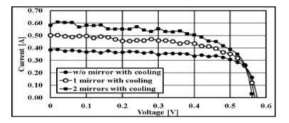
Figure 10. The I-V curve of solar cell with mirror and cooling
