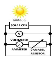
Figure 3. The measurement of solar cell
