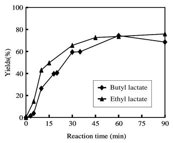
Figure 4. Effect of reaction time on production of lactic acid esters at 260°C.
