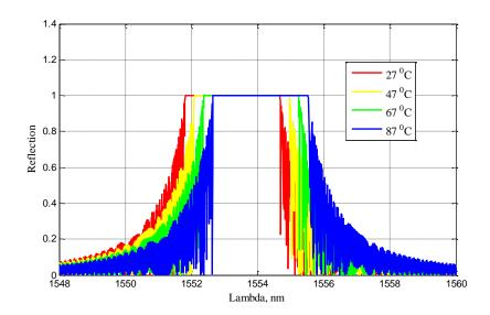
Figure 6. Temperature Effect on Uniform FBG (Method 2)
