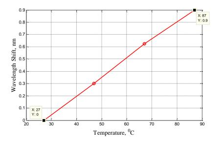
Figure 5. Wavelength Shift versus temperature (Method 1)
