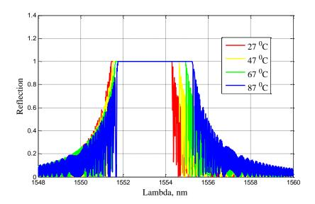
Figure 3. Temperature Effect on Uniform FBG (Method 1)
