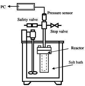
Figure 1. Schematic diagram of batch reactor apparatus.
