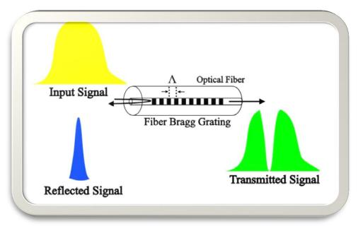
Figure 1. Schematic diagram of structure and spectral response of FBG, adapted from theory in Development of Fiber Bragg Grating Based Temperature Sensor System.
