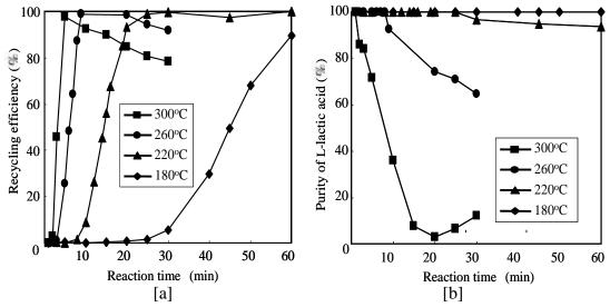
Figure 2. Effect of reaction time on recycling efficiency and the purity of L-lactic acid produced at various temperatures (sample: LACTY 5000).
