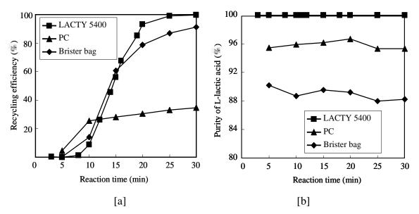
Figure 3. Recycling efficiency and the purity of L-lactic acid obtained from commercially PLLA product of brister bag and PC at  $220^{\circ}$ C and 30 min of reaction time.
