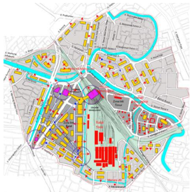
Figure 14: The proposed master plan of Manggarai District using Transit Oriented Development's concept Source: Dinas Tata Ruang DKI
