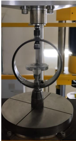
Gambar 2.1: Alat ukur gaya ( Proving Ring )
