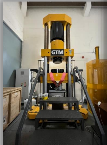
FORCE STANDARD MACHINE (GTM) 5 kN - 5 MN
