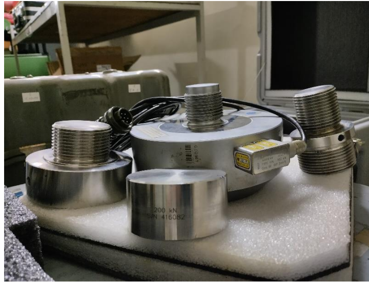
Gambar 2.1: Alat ukur gaya ( Load Cell )
