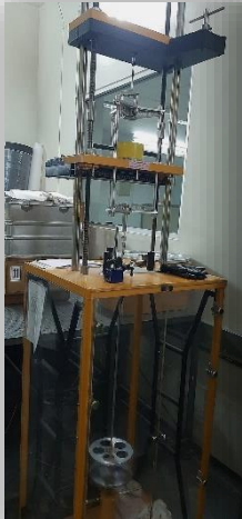
FORCE STANDARD MACHINE (KIM LIPI) 100 N - 1 kN
