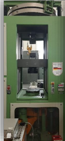
FORCE STANDARD MACHINE (SCHENCK) 2 kN - 1 MN
