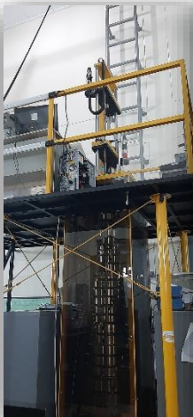
FORCE STANDARD MACHINE (GTM) 0.2 kN - 20 kN
