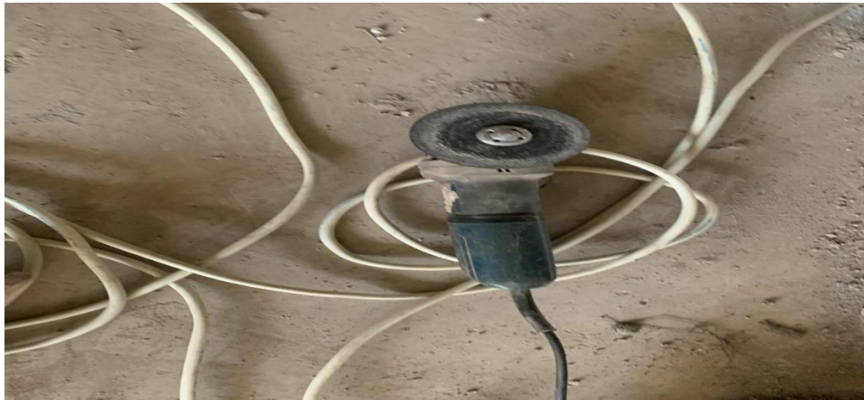
Gambar 4. 12 Gerindra Tangan ( Anglee Grinder )
