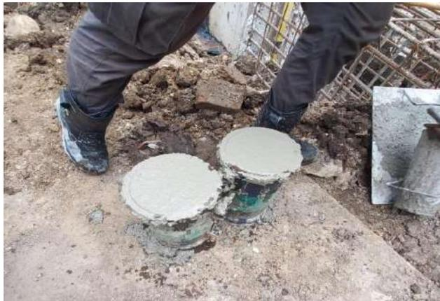
Gambar 5.9 Sampel beton silinder
